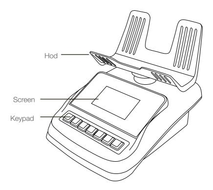
The Cashmaster Sigma 105 shown above is the device you are going to use. There are three main component parts:
